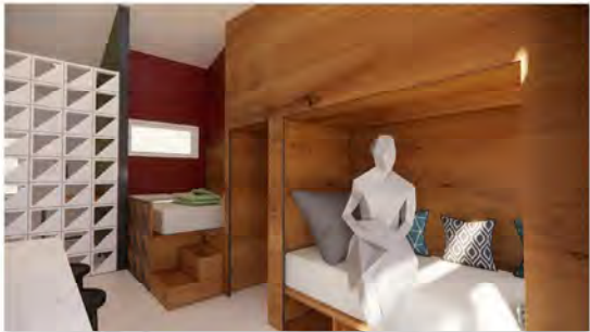
REST PLYWOOD JOINERY PROVIDES SPACES FOR SLEEPING AND RELAXING. PART OF THE JOINERY CONTAINS THE SAME PATTERN AS THE SCREEN.
